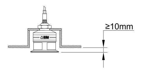
PTU50-51-56 can be installed in an extension pipe to turn away the sensor from the maximum level point. The extension pipe must be flat and without joints (welds, etc..), also, the pipe terminal part must be cut at 45° and with the borders without burr.
